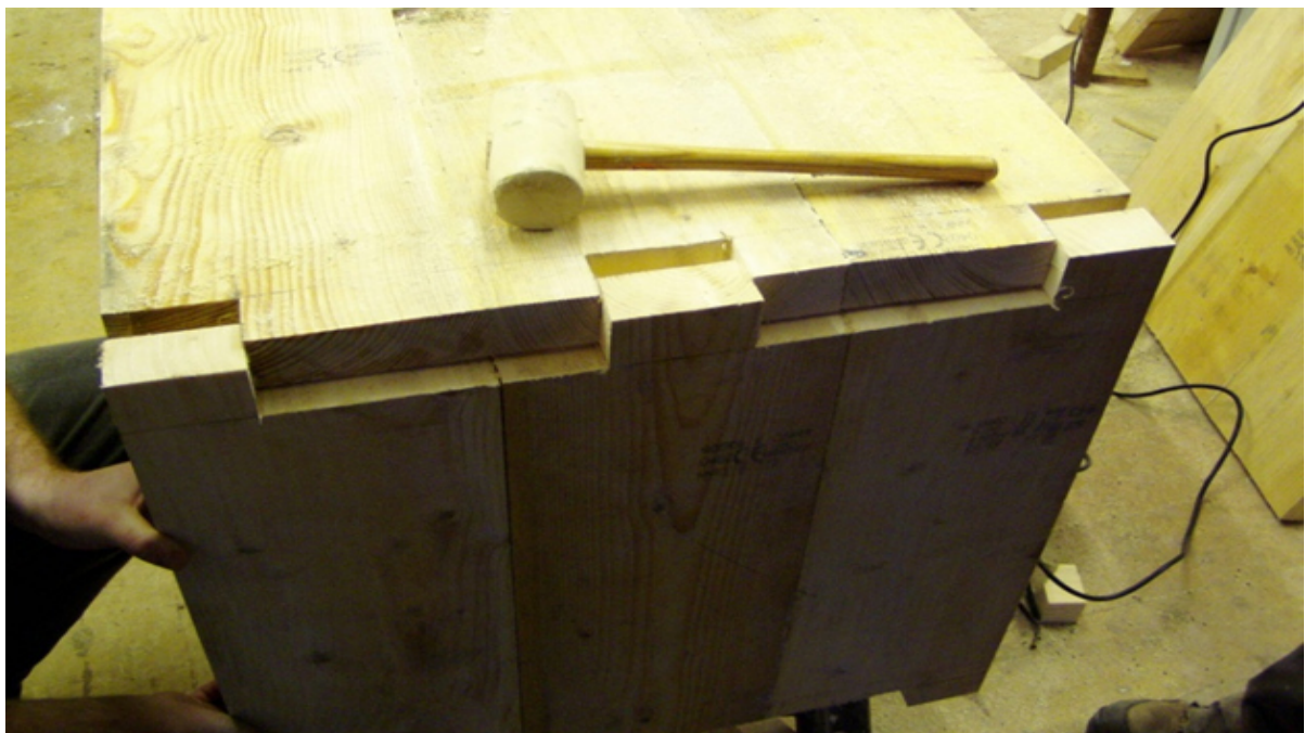
Plate 2: Traditional box joints used to construct wooden trough.
