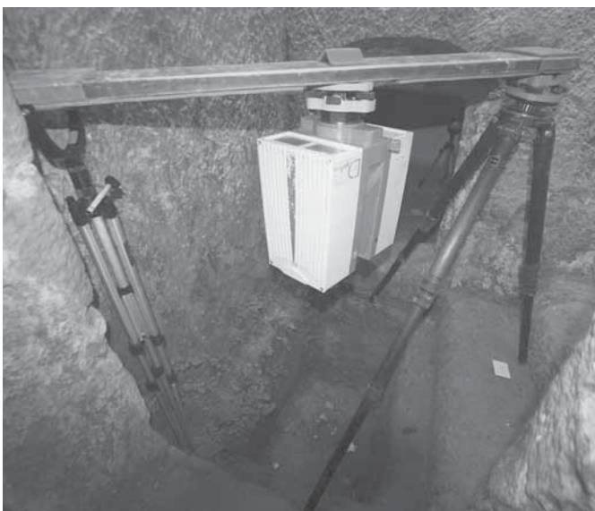
Fig. 4 An example of device used to solve the problem of surveying in small and narrow spaces.
