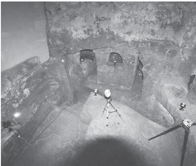
Fig. 3 Use of flat or spherical targets to ensure a good reliability of the survey.
